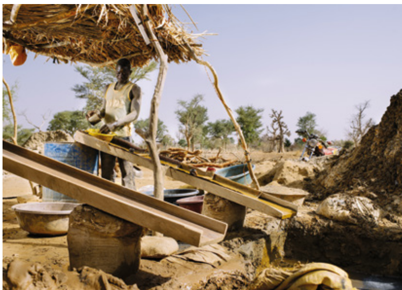
↑ A gold prospector uses a sluice box to filter the gold, Burkina Faso.
